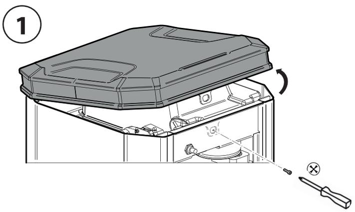
APRIRE IL COPERCHIO E ACCEDERE ALL'INTERNO DELLA BARRIERA PER LA RIMOZIONE DEGLI SPORTELLI / OPEN THE COVER AND ACCESS INSIDE THE BARRIER TO REMOVE OF THE DOORS / OUVRIER LE COUVERCLE POUR POUVOIR ACCÉDER À L'INTÉRIEUR DE LA BARRIÈRE ET RETIRER LES PORTES / ÖFFNEN SIE DIE ABDECKUNG UND GREIFEN SIE AUF DIE INNENSEITE DER SCHRANKE ZU, UM DIE TÜREN ZU ENTFERNEN / ABRIR LA TAPA Y ACCEDER AL INTERIOR DE LA BARRERA PARA RETIRAR LAS PORTEZUELAS
