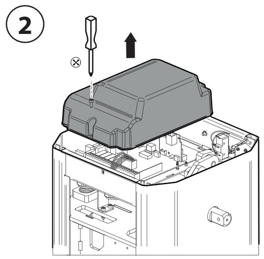
RIMUOVERE IL COPERCHIO DELLA CENTRALINA INTERNA / REMOVE THE COVER OF THE INTERNAL CONTROL UNIT / RETIRER LE COUVERCLE DE L'UNITÉ DE COMMANDE INTERNE / ENTFERNEN SIE DIE ABDECKUNG DER INTERNEN STEUEREINHEIT / RETIRAR LA TAPA DE LA CENTRALITA INTERNA.
