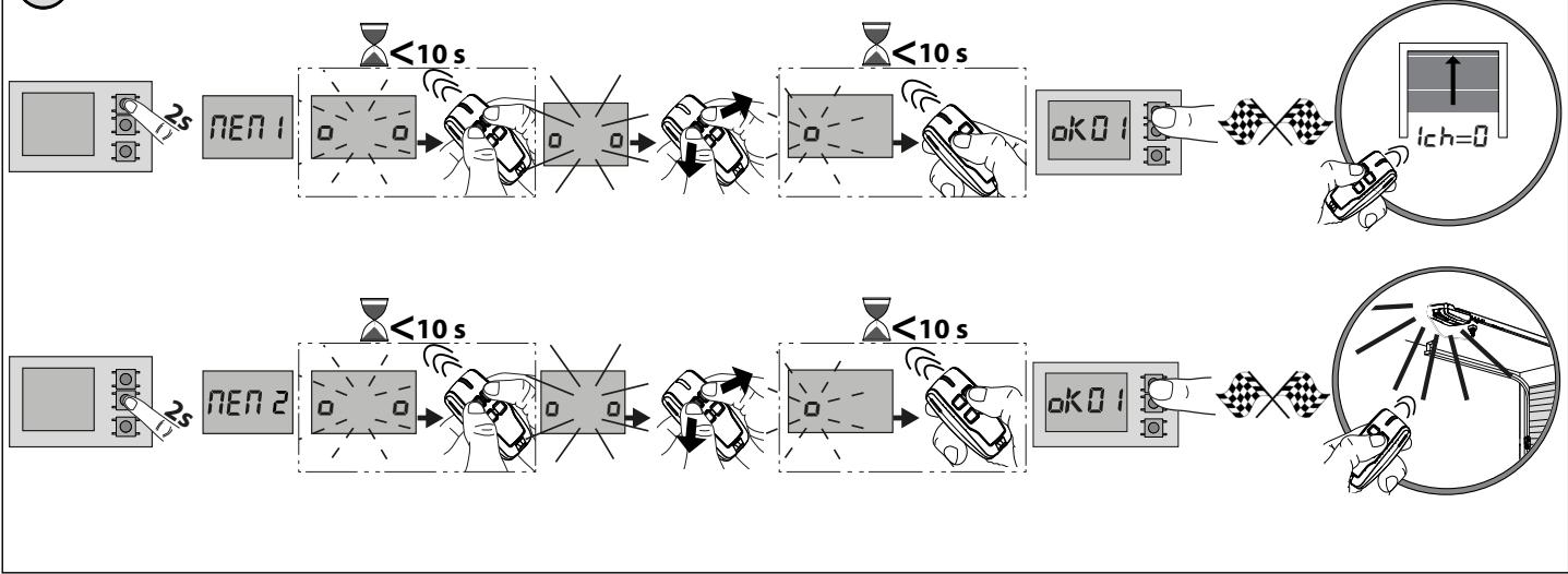
**P PROGRAMMAZIONE TRASMETTITORI REMOTA - REMOTE TRANSMITTER PROGRAMMING - PROGRAMMATION ÉMETTEURS À DISTANCE**
