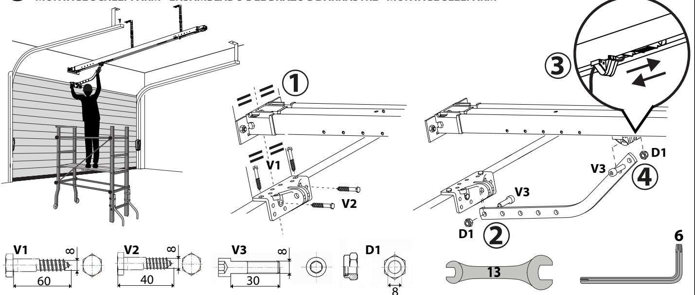
**G MONTAGGIO TESTA A BINARIO - HEAD ASSEMBLY TO RAIL - MONTAGE TÊTE À RAIL - MONTAGE KOPF AN GLEIS
