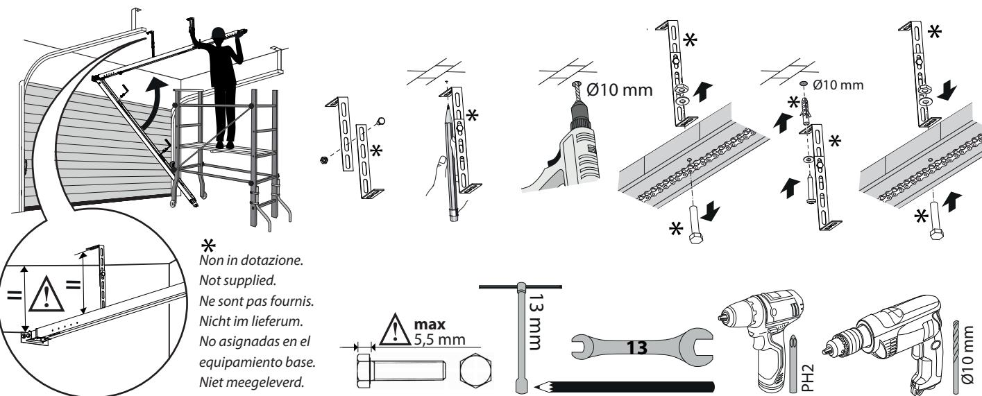
**F ASSEMBLAGGIO BRACCIO TRAINO - ASSEMBLY OF TRACK ONTO THE TRACK HOLDING BRACKET - ASSEMBLAGE BRAS ENTRAINEMENT
