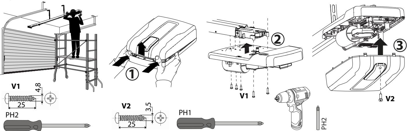
**H INSTALLAZIONI PARTICOLARI CON TESTA RUOTATA - PARTICULAR INSTALLATIONS WITH ROTATED HEAD- INSTALLATIONS PARTICULIÈRES AVEC TÊTE TOURNÉE-BESONDERE INSTALLATIONEN MIT GE SCHWENKTEM KOPF-INSTALACIONES ESPECIALES CON CABEZAL GIRADO-BIJZONDRE INSTALLATIES MET GEDRAAIDE KOP**
