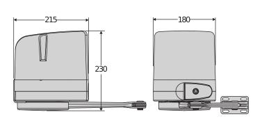
Electromechanical operator with articulated arm for residential use, for swing gate leaves of up to 2 metres and 200 kg. Ideal for all installation situations, with a lever system for the simple resolution of problems linked to large-size pillars. Control unit. limit switches and mechanical stops incorporated in operator.
