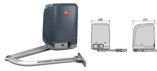
Electromechanical operator with articulated arm for residential use, for swing gate leaves of up to 2 metres and 200 kg. Ideal for any installation requirements, makes it easy to solve problems linked to large pillars thanks to the lever system. Operator-integrated control unit, limit switch and mechanical stops.
