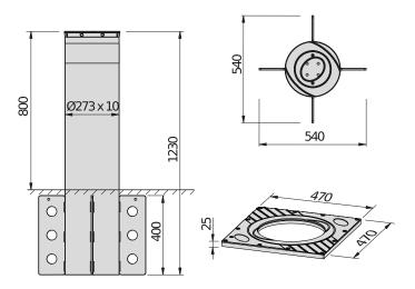
Permanent anti-terrorism bollard tested according to international standards PAS 68:2010 7500/50/N2 crash simulated. Suitable for protection of sensitive sites.
