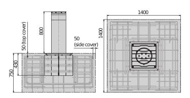
Permanent anti-terrorism bollard tested according to international standards PAS 68:2010 7500/50/N2 crash simulated. Suitable for protection of sensitive sites.
