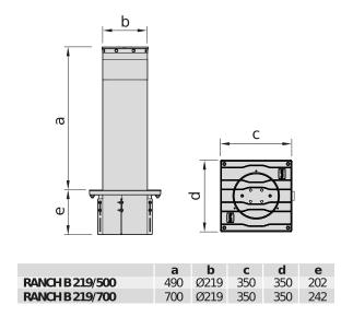
Fixed bollard, diameter 219 mm, used for long-term access prevention. Can be combined with automatic or semi-automatic bollards.
