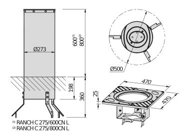
Fixed bollard, diameter 273 mm, used for long-term access prevention. Can be combined with automatic or semi-automatic bollards.
