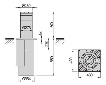
Automatic high strength anti-terrorism hydraulic bollard with incorporated hydraulic control unit. Suitable for protecting sensitive sites, thanks to the special "SD" version, which keeps the shaft raised in case of a power failure and with public installations where, in the standard version, the shaft lowers automatically when the power is cut.
