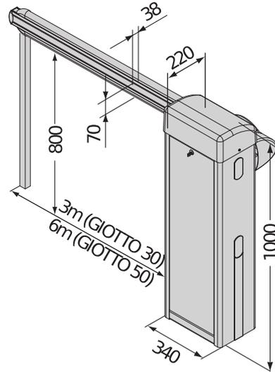
Range of barriers for intensive and very intensive use, able to manage useful passages up to 6 m. Integrated control unit with U-Link connectivity. Available in 24V versions, they have a wide range of accessories making them ideal in any context.
