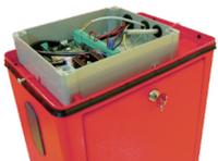
Control unit located in an easily accessible position and separate from the mechanical part
