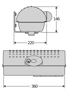
Range of 230V electromechanical operators for industrial folding doors, up to 2 panels per gate. Available also in 24V version to guarantee maximum anti-crushing safety and precision in movement and slowdown.
