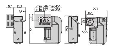
Electromechanical operator for semi-intensive use, for automation of industrial sectional doors up to 25 m² (Pegaso B Cja 625) or up to 45 m². Max. opening speed 24rpm and max. torque 70Nm (Pegaso B Cja 645). Dead man switch
