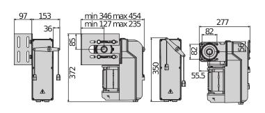
Electromechanical operator for semi-intensive use, for automation of industrial sectional doors up to 25 m² (Pegaso B Cja 625) or up to 45 m². Max. opening speed 24rpm and max. torque 70Nm (Pegaso B Cja 645). Limit switches with absolute encoder, with the possibility of rapid adjustment from floor.
