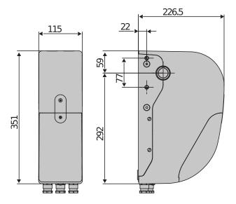
24V electromechanical operator for sectional garage doors installable in residential, industrial and commercial environments. The sturdy mechanical structure and microprocessor technology of the control unit make it possible to use the operator intensively whilst ensuring maximum reliability over time.
