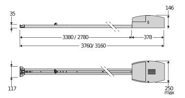
Electromechanical operators for intensive/very intensive use, designed for the automation of sectional garage doors. Suitable for installation in any context, thanks to the wide choice of chain rails available in the various lengths. The control unit and limit switch with encoder with mechanical stop are incorporated in the operator and rail respectively.
