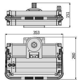
Low voltage hydraulic operator for very intensive use, suitable for any type of residential, industrial or multi-residence application. Compact and sturdy, they can automate swing gate leaves up to 2.5m wide and weighing up to 800kg.
