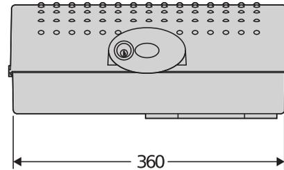
Range of irreversible electro-mechanical 24 v operators for swing gates up to 250 kg in weight and up to 2.5 m in length. Ideal for installation on large-size pillars thanks to its articulated levers that allow opening up to 125°.
