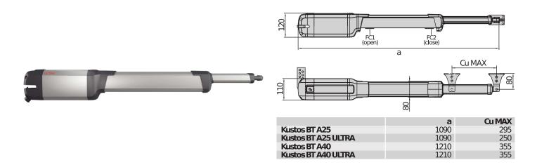
Complete range of electromechanical pistons for residential use, suitable for swing gate leaves up to 4 metres wide and weighing up to 500 kg. Quick and practical installation: the new KUSTOS BT A operators are designed to allow quick and easy installation, thanks to a number of important measures such as the covered worm screw, integrated stops, magnetic limit switches and the magnetic locking pin.
