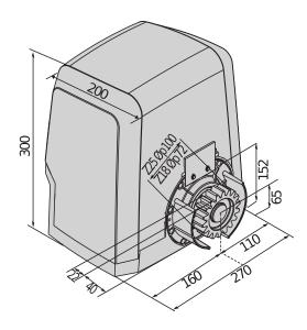
24 V operator for sliding gates weighing up to 1,500 kg, for intensive use. Maximum panel speed up to 12m/min. Torque control thanks to D-Track technology. Magnetic limit switches for quicker installation, more precise and better integrated with the architecture of site. Control unit with display, preconfigured for communication with U-Link protocol. Residential and commercial use.
