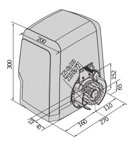
24 V operator for sliding gates weighing up to 1,500 kg, for intensive use. Maximum panel speed up to 12m/min. Torque control thanks to D-Track technology. Electromechanical limit switch. Control unit with trimmer and dip-switch. Residential and commercial use.
