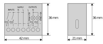
Miniaturized 2-channel indoor receiver for wireless control of lights or operators
