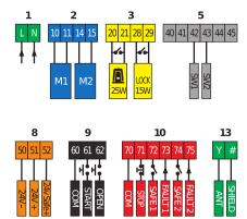
Control panel with dip switches and potentiometers for one or two 24V electromechanical operators for 230V/80W swing gates. The dual-channel radio receiver is incorporated.
