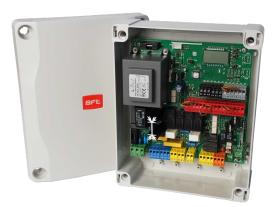
Universal control board with display for one or two swing or sliding door operators, 230V - 650+650W.
