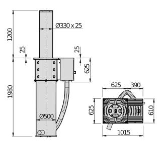
Automatic hydraulic anti-terrorism bollard, tested and certified (crash-tested) by independent body in accordance with standards IWA14-1:2013 and PAS 68, suitable for protecting sensitive sites. Independent hydraulic control unit for each bollard: if one control unit breaks, the other bollards will continue to function whilst maintenance work is facilitated.
