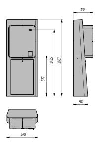
The ESPAS 20-P is a stand-alone automatic POF machine for Parking systems working without operator. It allows the programming of customisable rates
