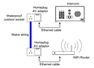
Note: The router needs to be on the same trip device as the power to the intercom for this technique to work. Always consult a professional electrician regarding mains wiring.
