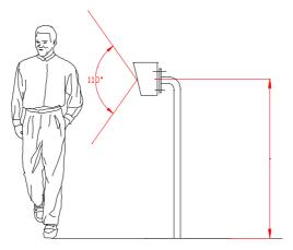
Mount the intercom at the desired height for pedestrian or car users. The camera angle is wide at 110 degrees to cover most scenarios.
