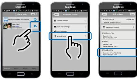
Check that the network which it is connected to is showing at least 20% strength. If it is not connecting, or is lower than 20%, then corrective action must be taken at this stage. Suggestions are as follows..
