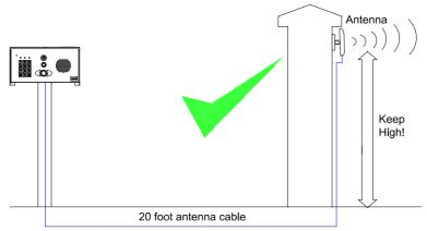
2. Change antenna angle slightly then re-scan the WiFi strength as shown above to check for improvements in strength. If signal improves, then continue to make small adjustments to the antenna angle and pitch to maximise strength.
