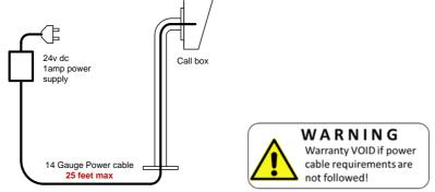
TIP: Most technical calls received are due to installers using thin gauge cable over longer cable runs. This intercom has a peak current demand of up to 2 amps.
