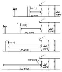
4. If it is not possible to have the WiFi router at the front of the building, then consider installing a standard "on the market" WiFi repeater or ranger extender. These can be purchased as a plug in device and are sold in DIY and consumer electronics stores.
