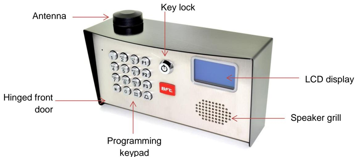
Any phone which receives a call from the intercom can activate a built in relay, which can be connected to an electric door release or automatic gate system.
