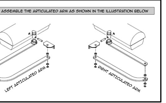
LEFT-SIDE OPERATORS - KEEP IN THE FULLY CLOSED POSITION RIGHT-SIDE OPERATORS - MANUALLY OPEN TO THE DESIRED LIMIT. CONTINUED ON OTHER SIDE...
