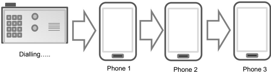
Any user receiving the call can answer, speak to the visitor, and press the following digits on their mobile or fixed line telephone to control the relay on the device...
