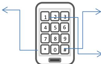
Press # key to **LATCH** output relay. Caution: Use only for holding open gates or door!.
