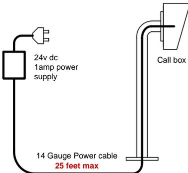
**Tip:** 18 gauge cable will not run the unit. You may experience various issues with performance if using 18 gauge or thinner, at more than 15 feet distance.
