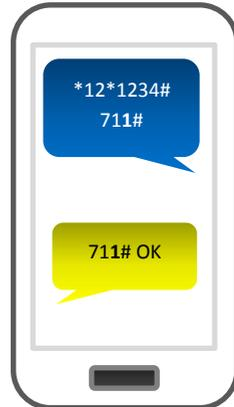
Now you may add numbers which can call the unit to trigger the relay by sending the following SMS (up to 3 phone numbers can be sent in a single SMS...)
