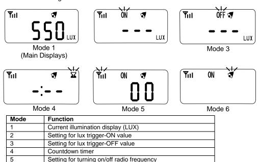
MODE 1 is showing as main display on the screen. Once mode setting is finished (MODE 2 to MODE 6), the screen will return to main display automatically after 12 seconds, or by pressing **ESC/** to return to main display.
