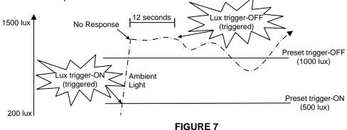
If no trigger-ON value is preset, to avoid the problem of consecutive triggering, the sensor has to be placed still for 2 minutes (restriction) before lux trigger-OFF is enabled again. To clear this restriction, the detected lux value of ambient light during this 2-minute period MUST be lower than the preset trigger-OFF value, otherwise the sensor will keep recounting the time before it can be triggered again (FIGURE 8).
