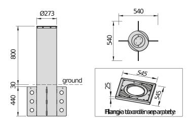
Fixed tall security bollard suitable for protection of sensitive sites. Reference standard PAS68:2010 7500/50/N2, ASTM2656:2007 M30. High-strength structure based on the design of the automatic version XPASS B 275/800.
