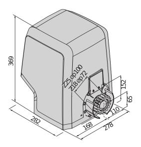
230V operators for sliding gates for very intensive use, extremely robust and high-performance thanks to oil bath transmission. Torque control thanks to D-Track technology and encoder for the highest possible precision of movement. Control unit for communication with U-Link protocol and with tamper-proof function. Operator with magnetic limit switch.
