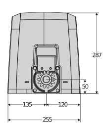
24 V operator for sliding gates weighing up to 600 kg, for intensive use. Maximum panel speed up to 16m/min. Torque control thanks to D-Track technology. Magnetic limit switches for quicker installation, more precise and better integrated with the architecture of site. Control unit with display, preconfigured for communication with U-Link protocol. Residential use.
