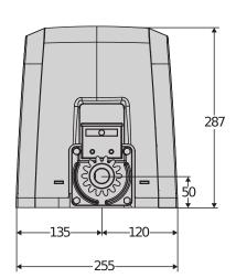
24 V operator for sliding gates weighing up to 600 kg, for intensive use. Maximum panel speed up to 16m/min. Torque control thanks to D-Track technology. Electromechanical limit switch. Control unit with trimmer and dip-switch. Residential use.
