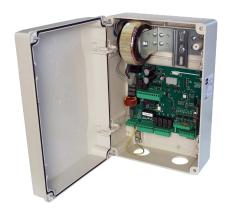
Control panel with display for one or two 230V used on electromechanical or hydraulic parking bollards. It can deal with up to four bollards simultaneously (or two in the case of the Xpass 1200 models) and has configurable outputs and a connector for a 433 MHz radio receiver with optional 2048 code memory.
