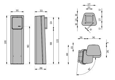
The ESPAS 30-U ULTRA station is a device for managing an exit gate from a parking area. The unit works in a wired network
