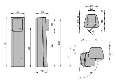
The ESPAS 20-U station combined with an electromechanical barrier is a device for controlling an exit transit point of a parking area. The system works in stand alone mode, and no wiring is required between the various components of the car park. It includes scanner for ticket and Proximity Card readers
