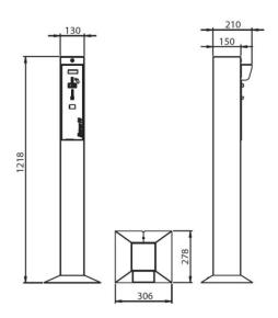
Entry/exit station for parking systems for collective use, able to operate in "stand-alone" mode. The unit provides entrance and exit control and can be connected to electromechanical barriers.
