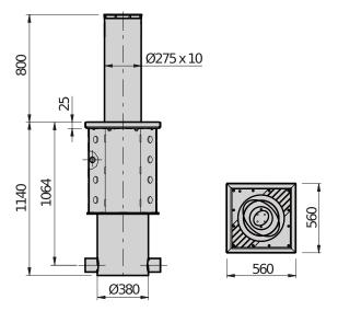
Automatic hydraulic anti-terrorism bollard, suitable for protection of sensitive sites, tested and certified (crash-tested) according to the IWA14-1:2013 standard with V/7200 [N2A]/48 rating, equivalent to PAS68:2013 with V/7500 [N2]/48, ASTM2656:2007 M30 rating. Double installation. Independent hydraulic control unit for each bollard: if one control unit breaks, the other bollards will continue to function whilst maintenance work is facilitated.
