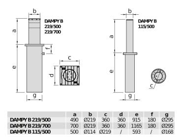
Semi-automatic bollard driven by gas spring for controlling road access points. Competitive and easy to use. Also available with stainless steel shaft and light cap.
