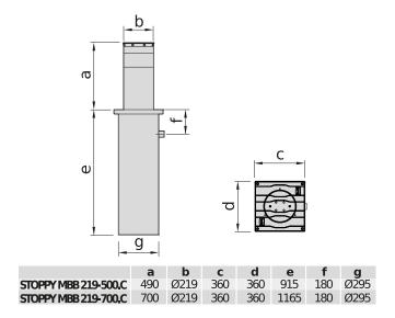
Retractable electromechanical bollard for safety and protection in all areas that require controlled access.
