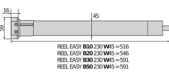
The Reel range consists of a complete offer of wire tubular motors, with electromechanical limit switches.
