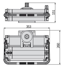
Low voltage hydraulic operator for very intensive use, suitable for any type of residential, industrial or multi-residence application.
