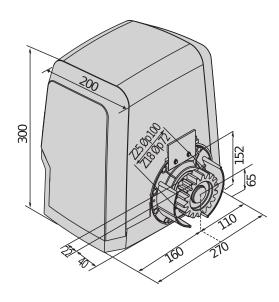
24 V operator for sliding gates weighing up to 1,500 kg, for intensive use. Maximum panel speed up to 12m/min. Torque control thanks to D-Track technology. Magnetic limit switches for quicker installation, more precise and better integrated with the architecture of site. Control unit with display, preconfigured for communication with U-Link protocol. Residential and commercial use.
