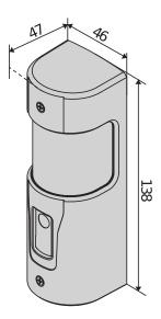
Wired or wireless adjustable photocells with maximum range 30 m.
