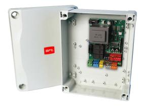
Control panel with dip switches and potentiometers for one or two 230V/500W operators used on sliding and swing gates, shutters and overhead doors with the management of up to two sensitive edges (one of which type 8K2).
