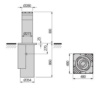
Automatic high strength anti-terrorism hydraulic bollard with incorporated hydraulic control unit. Suitable for protecting sensitive sites, thanks to the special "SD" version, which keeps the shaft raised in case of a power failure and with public installations where, in the standard version, the shaft lowers automatically when the power is cut.
