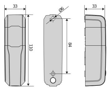
Pair of adjustable photocells, designed to offer a high level of installation flexibility thanks to their compact size, the possibility to adjust the head by 90° horizontally, left and right (180° in total), and a wide input power supply range 12-33Vac and 15-35Vdc. 20 metre nominal range.
